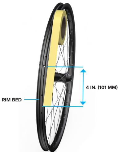
3. Hold your thumb firmly over the adhered end of the tape against the rim. Rotate the rim forward so that the free length of tape is in line with the adhered section of tape. This will allow you to apply correct force, or tension, on the tape.
