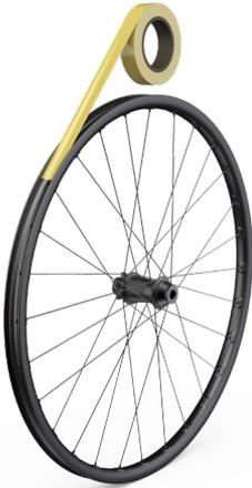
4. Adhere the tape by maintaining tension on the tape and firmly pressing it down onto the rim in short sections with your thumb. Continue this technique around the circumference of the rim until you reach the starting point of the tape (not pictured).
