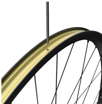
2. Install the valve stem through the rim tape and into the valve stem hole. Thread the nut onto the valve stem from the opposite side of the rim.
